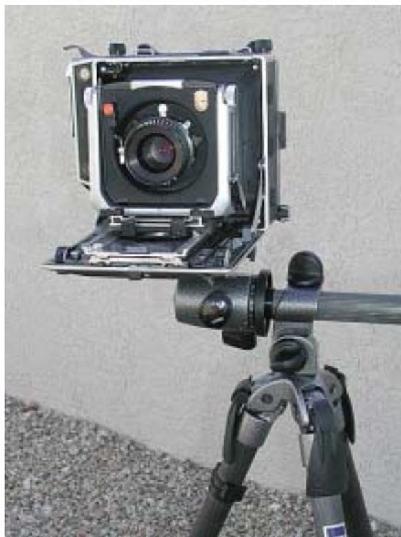
Linhof 4x5 mounted sideways and vertically on the tripod. Since the Linhof has a rotating back it is possible to take both vertical and horizontal view with this setup.
