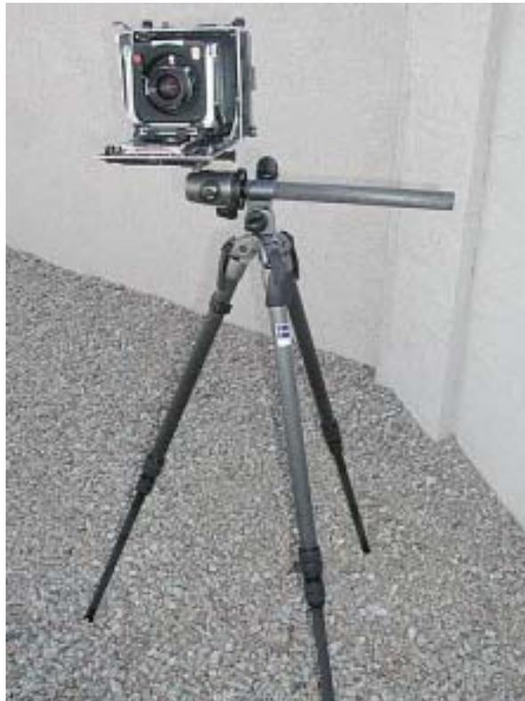
Linhof Master Technica on sideways center column. Since the center of gravity is only off a couple inches from the actual center of the tripod this configuration is actually quite rigid and vibration free.
